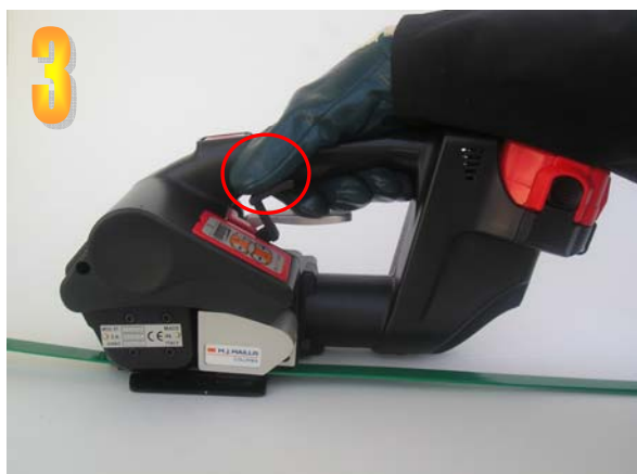
SEALING AND CUTTING PHASE
