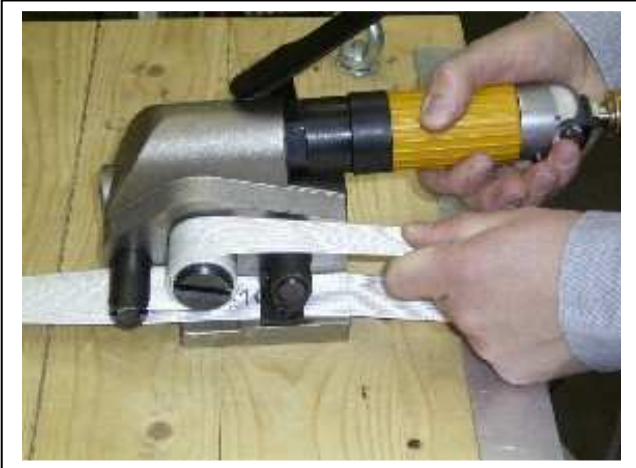
Tension the strap by pushing the button on the grip.
