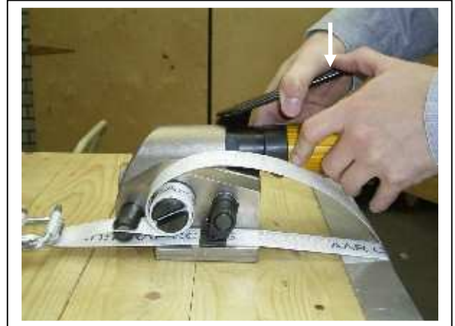
Upon completing squeeze the handle so cutting and releasing the strap. Move the tensioner away to the right.
